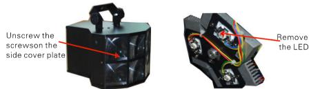
First, unscrew the screws on the side cover, then remove it, and unscrew the screws which on the LED board, then remove the LED board. If there are LED lamps were damaged, you need to use the thermostatic electric iron to remove it. Installation is in the opposite way.
