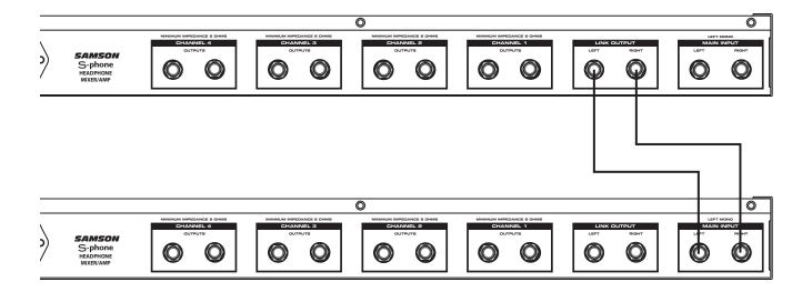
Because the S•phone Stereo Link output jacks are electronically balanced, we recommend the use of 3-conductor cable and 1/4" TRS (Tip/Ring/Sleeve) connectors. Even when several S•phones are linked together this way, there is no loss of power or audio fidelity—every Channel on every S•phone will sound just as loud and clear as if it were the only unit connected. The status of the front-panel Stereo/2 CH buttons affects only that unit and has no effect on any subsequent linked units.
