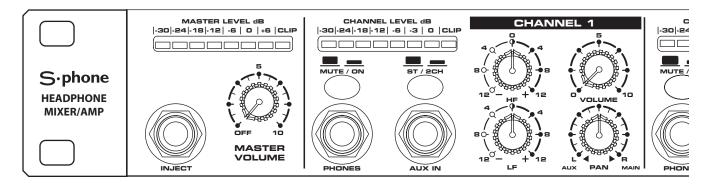
MASTER VOLUME – OFF CHANNEL 1 MUTE SWITCH – OUT CHANNEL 1 ST/2CH SWITCH – OUT CHANNEL 1 HIGH FREQUENCY – 0
