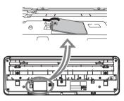
3 Insert the six new batteries, being careful to follow the polarity markings on the inside of the compartment.
