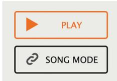
The Play button at the center lets you start the HW sequencer when the MIDI SYNC settings are set to EXT or USB (letting you send the MIDI Clock from the Editor to the hardware unit). This normally starts and stops the playback of the loaded pattern, but when in SONG MODE it will start and stop the playback of the song.
