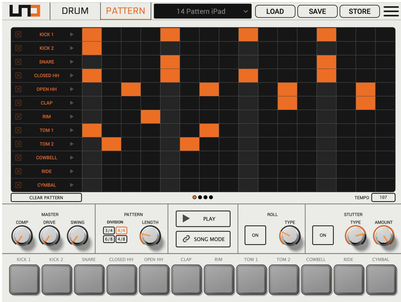
The pattern panel is where the features of the powerful UNO sequencer are shown. Here it is possible to create and modify patterns, and/or automate all the parameters of all the elements, per step up to 64 step, then save it where you prefer and load it whenever you want.
