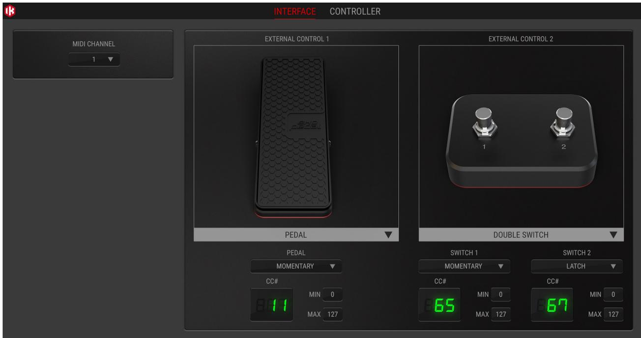
The Controller tab gives you control over the 2 controller inputs. Set behavior, MIDI channel, MIDI CC#, minimum and maximum values, and more, to dial in the best settings for whatever application you want to control.
