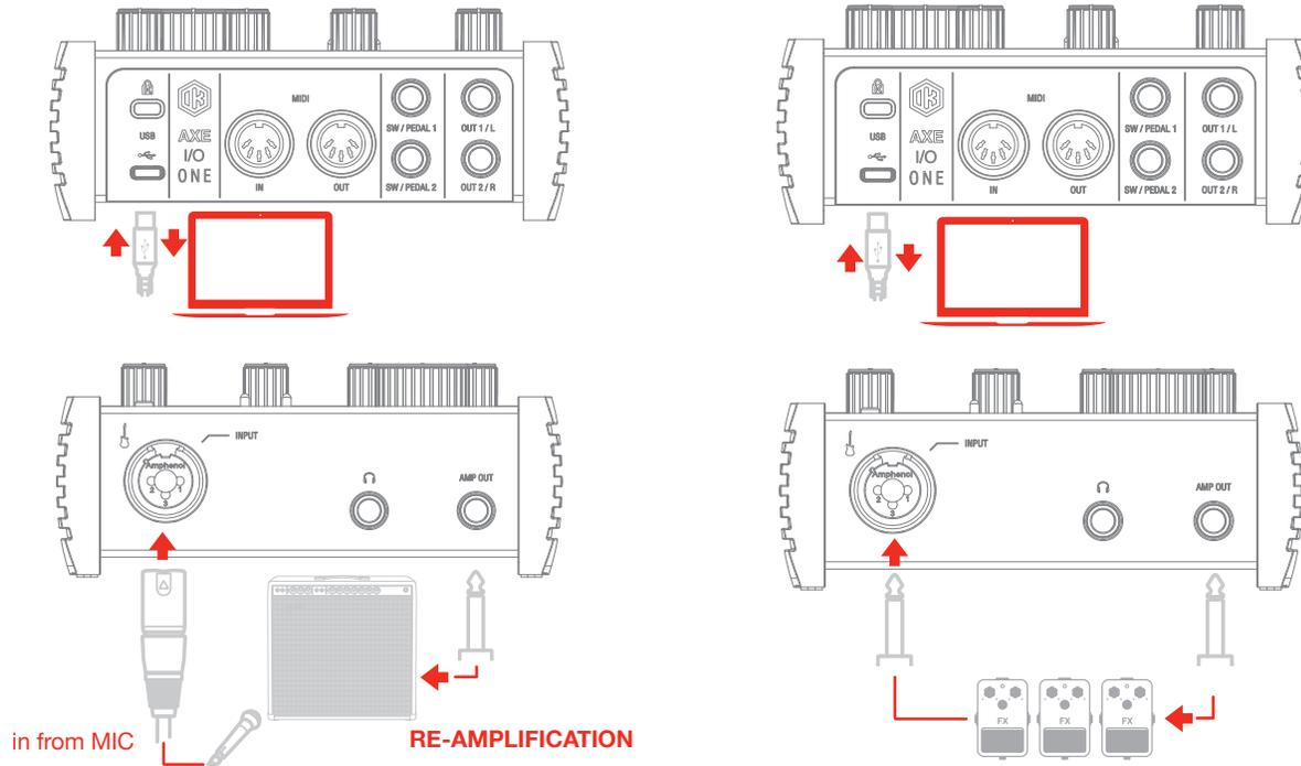
Among the features that make AXE I/O ONE the definitive guitarist interface is the re-amplification feature. The “AMP OUT” is a third physical output which is independent from main Output 1-2. With this output, you can feed a DI recorded guitar to external analogue stumps or a real amplifier, still being able to monitor the session from main Output (1-2). The external stumps (or the miked amplifier) will be connected back to Input to return into the DAW on a newly recorded track.
