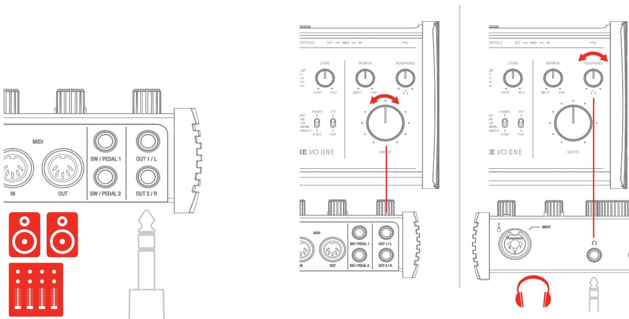
The 1/4" jack outputs 1/L and 2/R on the rear panel will normally be used to drive monitor speakers. Self-powered (active) monitors incorporate internal amplifiers, and may be connected directly. Passive loudspeakers will require a separate stereo amplifier; in this case, the rear panel outputs should be connected to the amplifier's inputs.
