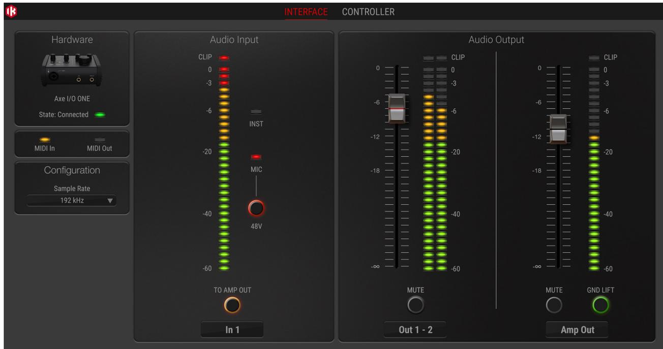
**State.** This LED shows when an AXE I/O ONE unit is connected and active.
