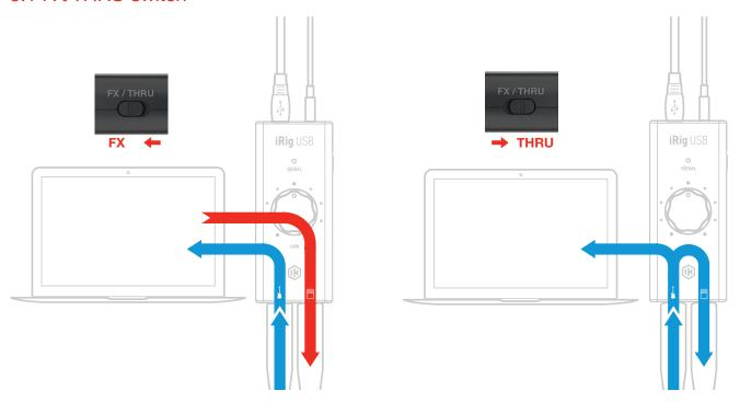
The THRU-FX switch allows you to select the type of output that is sent thru the "Amplifier output jack."
