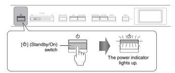
3. Press and hold the [O] (Standby/On) switch for a second to turn the power off.
