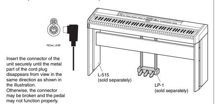
Make sure that power is off when connecting or disconnecting the pedal unit.
