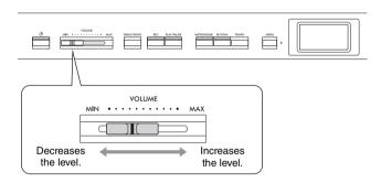
Adjusting the [VOLUME] slider also affects the output level of the [PHONES] jacks (page 14) and the output level of the AUX OUT jacks (page 76).
