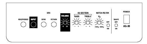
**HEADPHONES:** This jack provides a stereo signal to drive headphones. The use of this jack will disengage the amplifiers internal speaker. **INPUT:** Instrument input. Designed for both active and passive pickups.
