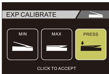
3. Set the pedal in the toe down position and apply forward pressure. Whilst applying forward pressure, press the VALUE control to confirm. This will set the sensitivity of the EXP pedals toe down activation switch
