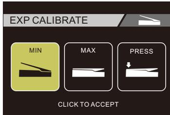
1. Set the pedal in the heel down position and press the VALUE control to confirm
