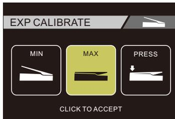
2. Set the pedal in the toe down position and press the VALUE control to confirm
