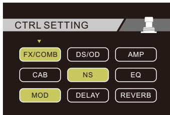
Use the VALUE control to highlight and select which effects blocks you wish to assign to be switchable using the CTRL/TAP footswitch.
