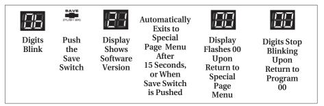
After showing you the software version, the display will flash 00 to indicate you're back in the Special Page menu. You may now choose either a new Special Page function, or press **Save** again to exit. If you don't make a choice in about 15 seconds, the display stops blinking, indicating the SansAmp PSA is in Program 00, bypass.
