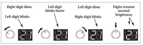
Assume the preset point for a particular knob is 12 o'clock. If the left digit blinks and the right dims after unlocking it, you will need to turn the knob clockwise to reach the preset value. As you get closer, the left digit will blink faster, then stop when you've reached the stored value. The right digit then resumes its full brightness. Conversely, if the right digit blinks and the left dims, you will need to turn the knob counter-clockwise, etc.
