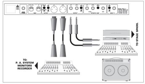
The SansAmp PSA has dual 1/4" unbalanced and XLR balanced Outputs for interfacting with all types of gear. XLR Outputs provide a signal for driving pro gear, including P.A. systems, mixers, signal processors. 1/4" Outputs are ideal for feeding most mixers, signal processors, and instrument amplifiers. Each set can be used simultaneously and independently.
