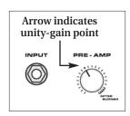
AFTER BURNER ZONE: The area where a low-cut/hi-boost function is activated. This gives more definition to individual notes when using high gain sounds. If buzzier, fuzzier sounds are desired, increase the gain by using the **Drive** control and set the **Pre-Amp** control outside the After Burner zone.
