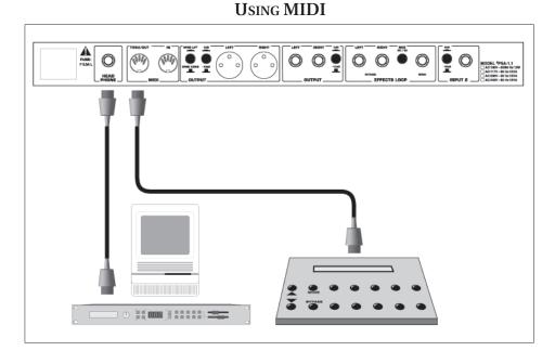
All MIDI gear, including MIDI footcontrollers, signal processors, keyboards, and computers, can be connected to the SansAmp PSA. The MIDI In accepts Program Change commands, as well as MIDI Map and Program dumps. The MIDI Thru/Out jack is usually configured as a MIDI Thru, succept when data is being transmitted from the SansAmp PSA.
