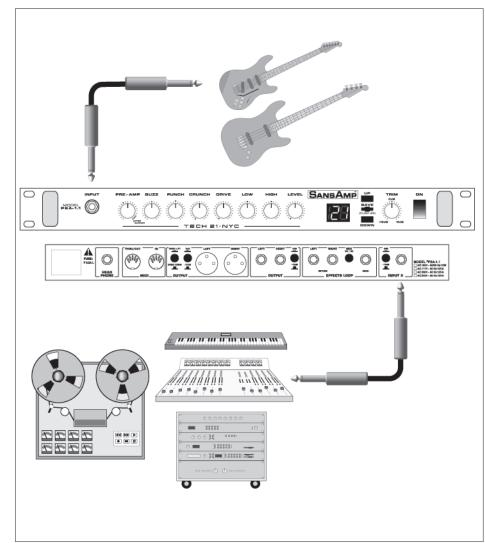
The front-panel Input jack is designed to accept signals from guitars, basses, keyboards, etc. You can set up your SansAmp PSA as a permanent part of a rack or patch-bay setup, with its usual input source plugged into the rear-panel jack. Then, if you want to plug straight into the SansAmp PSA, use the front-panel Input, which overrides the rear-panel Input 2.
