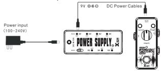
If the input polarity of the electrical device is , please connect polarity reversal cable to the DC power cable, then connect the device
